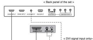
Connect the signal cable from the monitor output socket of the DVD player or Set top Box to the **HDMI INPUT** socket of the set.
